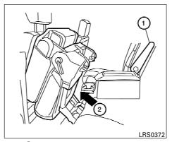
Then ② lift up on the lower corner of the seat base and tip the 2nd row captain's chair forward. To exit the 3rd row bench seat, lift up on the same seatback latch and fold the seatback forward onto the seat base. Then lift up on the seat base and tip it forward.
